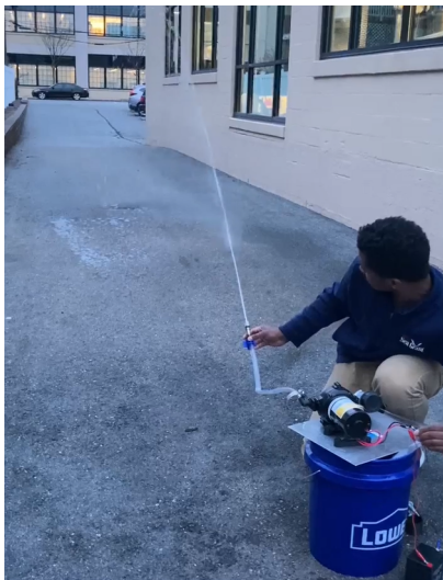
Fig. 13: Experimental water gun mechanism set up at MIT Sea Grant to determine trajectory of the water output.
